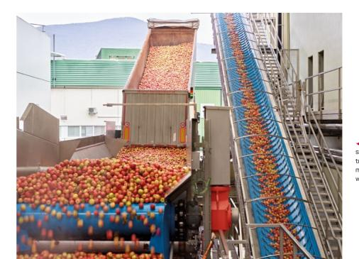
On the new receiving station apples are transported in a "dry" manner, which saves water.
